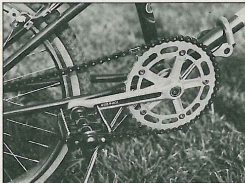
We chose DuraAce cranks with a 44:16 ratio. We used the Shimano chromemoly loose ball-bearing bottom bracket.
