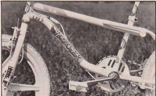
GT could almost have a circle-the-improvements contest with this photo. From left to right we have the new, shorter fork dropouts, trick through-the-frame cable routing, lower S-bend foot platform, and redesigned top platform. You definitely get your money's worth with this scoot.
