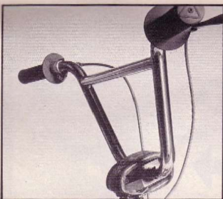
The GT Pro bars won points for their bend and width. They're a tad wider than most. These are a hot tip item for larger riders.
