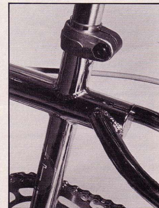
The seat tube piercing the extended top tube clearly identifies a GT. They pioneered this design.
