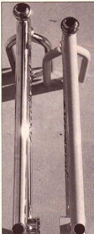
Both the Limo and the Pro have mini-gussets, and oversized 1-1/4-inch top and down tubes.
