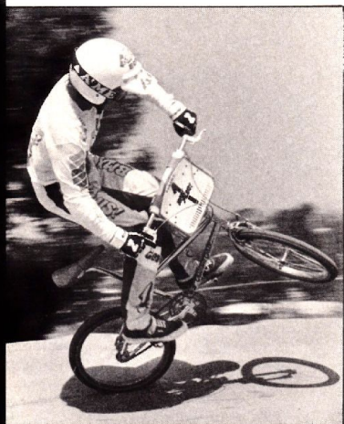
The short rear end makes the Super Viper wheelie really easily—maybe too easily. It might be worthwhile to switch to a straight seatpost to get your weight a little farther forward.
