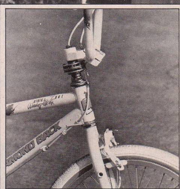
Not only did the ACS angled stem lower the bars for comfort and riding ease, the ACS brakes provide sure stopping.
