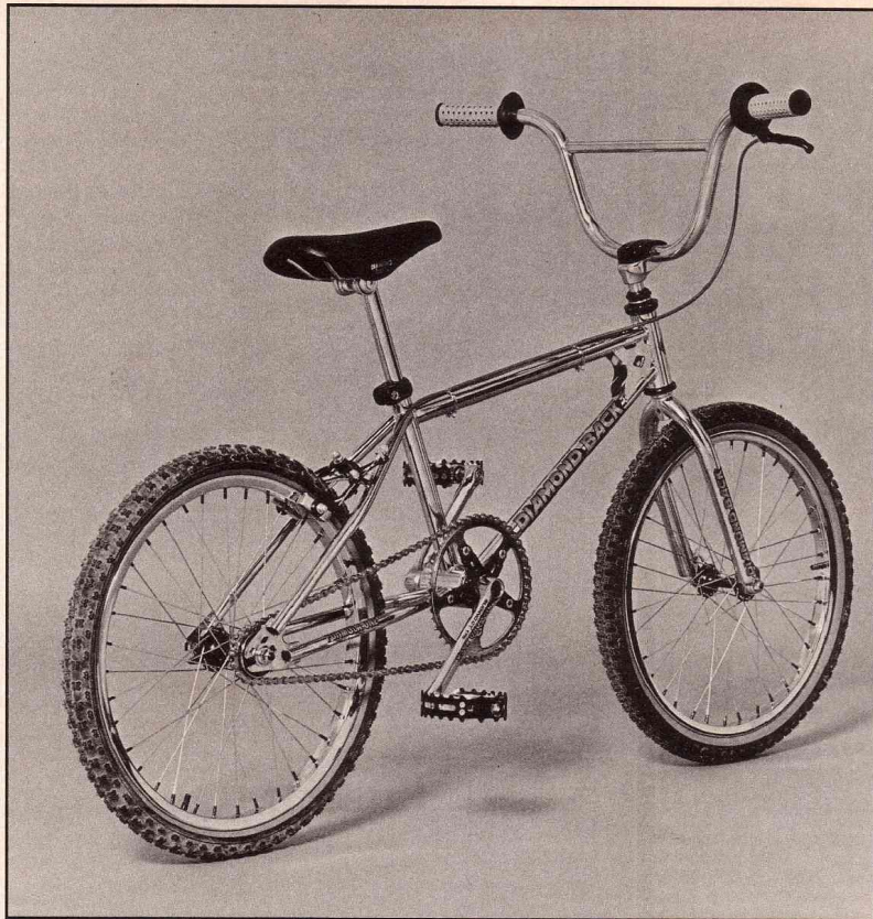
Diamond Back's Formula One. This is a mega-excellent crit craft for dudes in the 11-13 age range. Box stock it weighs in at a trim 21 pounds, 7 ounces, and there are a few simple areas like the seat and the cranks where you can EASILY chop a couple MORE pounds.
