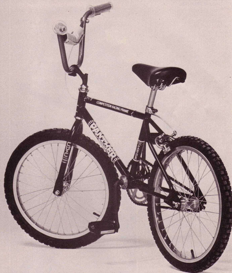
With a 73 degree steering head angle, 34 inch wheelbase, and 1 3 / 16 inch fork rake, this is a QUICK handling bike. And we do mean QUICK.
