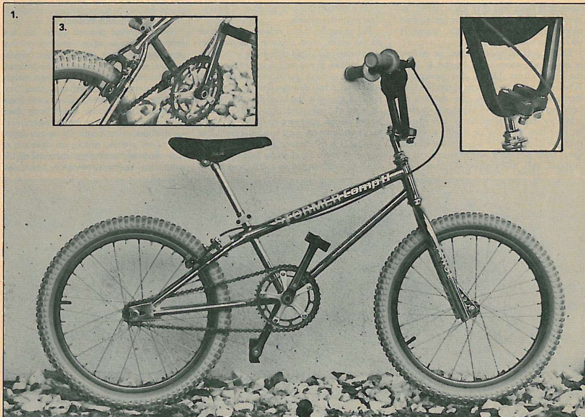
1. The Stormer Competition II comes to you courtesy of CYC, who also carries a big line of bike products. Check out the thick top tube and straight line geometry from the rear wheel. 2. Handlebars are quality alloy items which are held down by a massive aluminum and moly steering stem. 3. Single caliper brake is a Shimano side-pull. The crank is the trick Shimano 600 EX alloy with bizarre but functional plastic pedals by Kingsbury.
