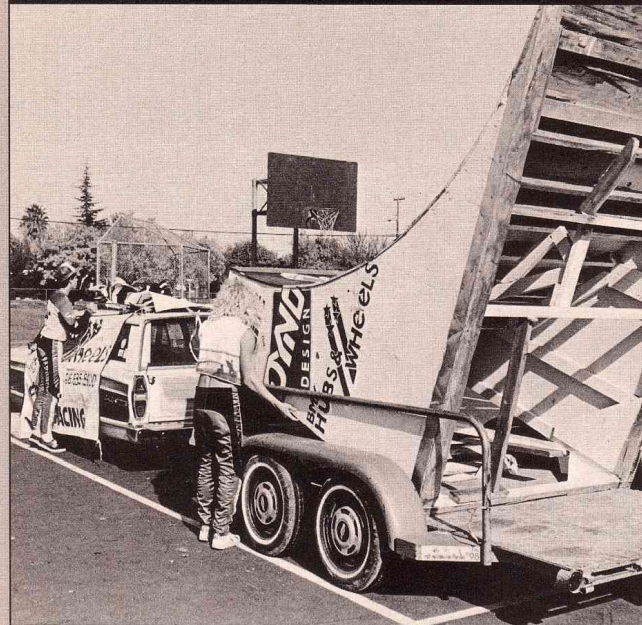
The Gork rig. The quarter pipe — "Big Boy" — was designed to fit into the trailer, making transportation a cinch. The small ramp tucks in underneath "Big Boy" at the front of the rig.
