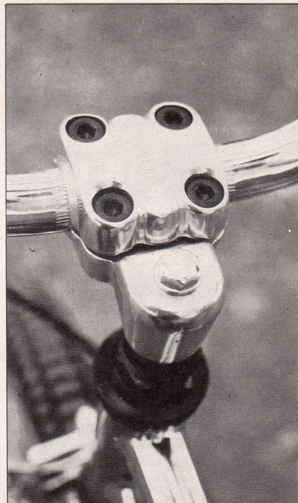
The Apollo's head stem. It's an alloy clamp job.
