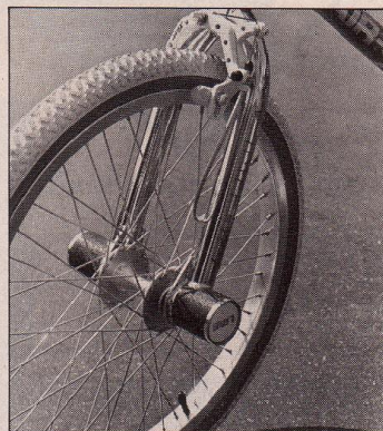
We had no problems with the alloy 48s or the Chang Shin tires, but the wheel did slip out of the dropouts on one occasion. Fortunately, the platforms kept the wheel intact, and they work good for standing, too.
