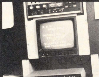
This is a character generator. Using this machine the producers can put just about any character over the image. Usually titles and credits are created using machines like this one.
