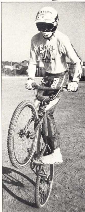
The frame and forks are made of 4130 chromoly.
