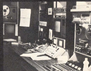
A look at the mixing room. The video tape recorders are located off the picture to the left. On the left is the character generator, in the center on either side of the telephone in the video mixing equipment and on the extreme right is the audio mixing equipment.
