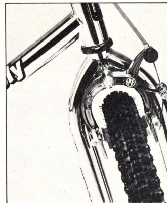
Brakes are by Dia-Compe, the Murray comes with a front and rear brake.
