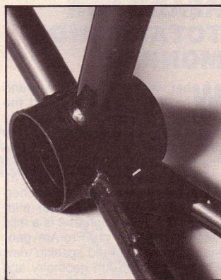
A double gusset bolsters the chain stays.
