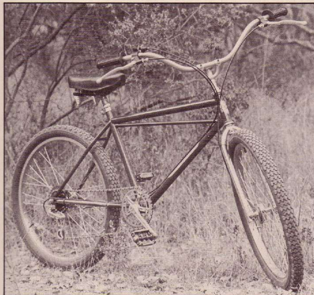
The Pro Cruiser: Chrome-moly frame, Tange forks, Shimano cranks, Mesinger seat, Ukal aluminum rims, stainless steel spokes, Carlisle Nobby tires, etc. 5 speeds. Cost is $500.
