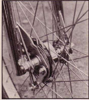
The Pro Cruiser runs Sturmev-Archer drum brakes front and rear.
