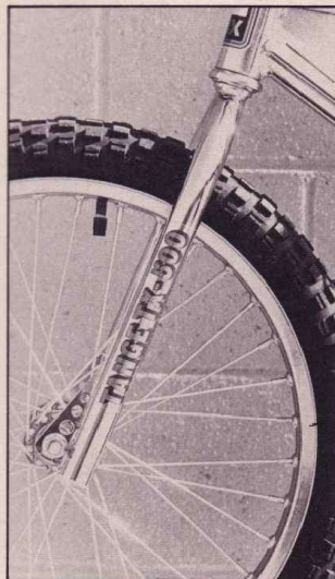
Tange TX-500 forks, Cheng Shin knobblies, 36/.105 spokes, Femco dimpled steel rims ... bulletproof equipment.
