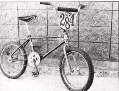
At first glance, Scot's '76 FMF doesn't look that different from today's bikes, except for the Addicks plastic sprocket, the Bendix coaster brake and the Huffy stem (it's hidden behind the numerplate).
