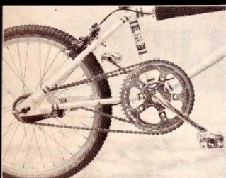
Power Plus Products was in Long Beach telling the world about its new X-2 transmission system. The X-2 operates using two chains. The shifter is operated by a lever traditionally used for brakes. For those of you who want to shift into the winner's circle, write Power Plus Products, 920 Gavler St., New Orleans, LA 70112-1602.
