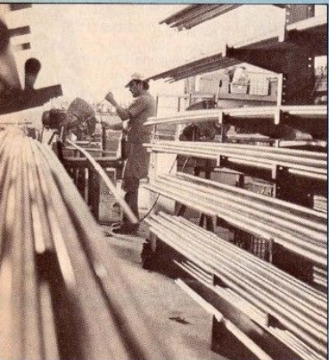
The first step in building a bike is cutting the tubing to the necessary lengths.
