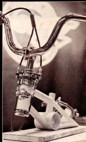
Odyssey was at the show displaying its new Gyro cable detangler. The Gyro operates with two cables to provide an even pull when you apply the brakes. It was designed by freestyle's mad scientist, Brian Scura. The best thing about the Gyro is that it will be considerably less expensive than the other detanglers on the market. For more info ask your local bike shop for Odyssey.
