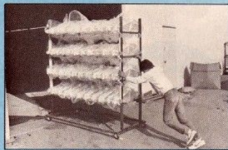
After inspection, GT sends the frames out for painting or chrome plating. This GT employee wheels a full rack of frames into the GT plant after they came back from the painter.
