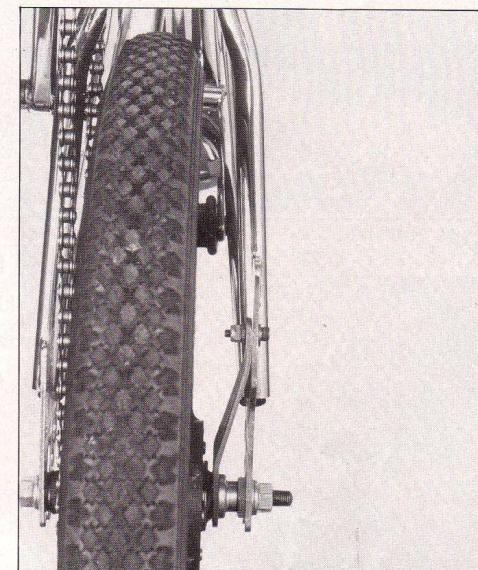
The SunTour coaster brake arm must be modified by bending it beneath the chainstay.
