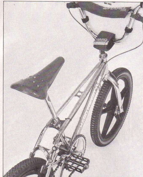
Topside view shows the studded pilot's seat and the double top tubes covered with clear 3M grip tape.
