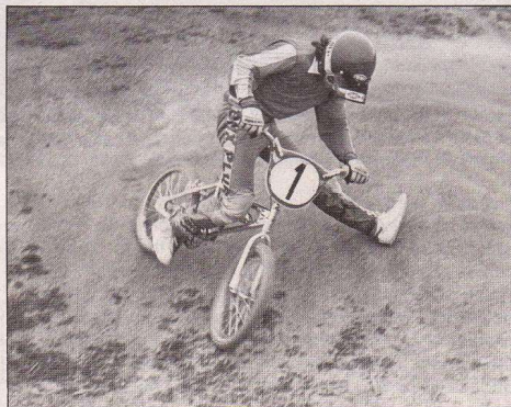
The Bridgestone doesn't plow into turns when the limit of traction is reached; instead it makes a smooth transition into a slide.
