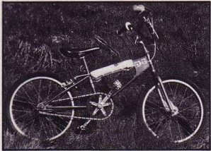
The Fleming machine: DG frame and forks, Dura-Ace cranks, Phil Wood hubs, Reedy pedals, Stronglight bottom bracket, Swallow 1.75 street tires, alloy bars, derailleurs alloy gooseneck, HKK chain, 42T front sprocket, 15T rear freewheel, Dia Compe calipers, Oury grips, Seamless YFC seat.
