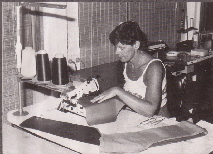
Sewing of the strong nylon BMX pants also requires strong threads, so commercial-style sewing machines are used. As they say in the sport 'your clothing is only as good as the seams.'
