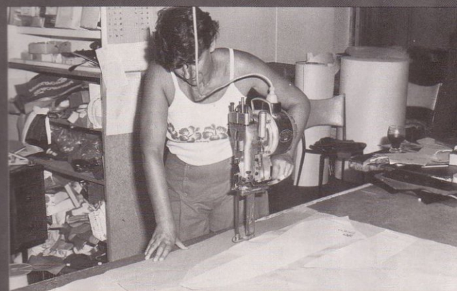
Jan Pearse handles the workshop of Peddle Power, often rolling up her sleeves and getting into the production side of things when the pressure is on. Here she uses a commercial material cutter to cut out the patterns for BMX pants.
